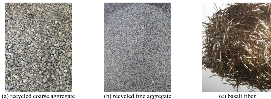
Figure 1 Schematic diagram of recycled aggregate and fiber
